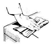
AFTER WASHING, use a soft dry cloth to wipe the outside and inside dry. Leave the lid up until the basket is dry. Wipe up spills right away. Spills can dull or damage the finish.
